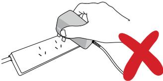
**Do not** connect your nbn™ connection box to a power point using an extension cable, double adaptor, power board or any other kind of secondary plug or socket.
