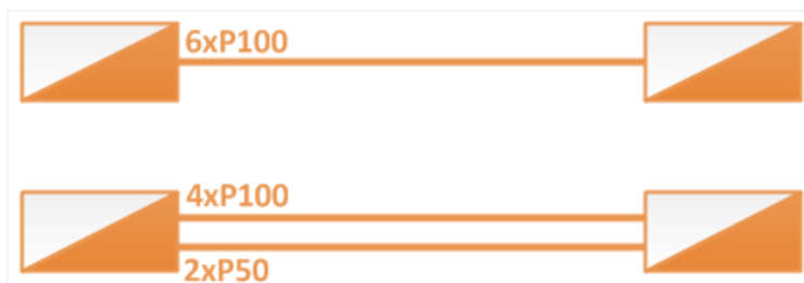
Figure 14. Distinct multiple conduits (manhole)
