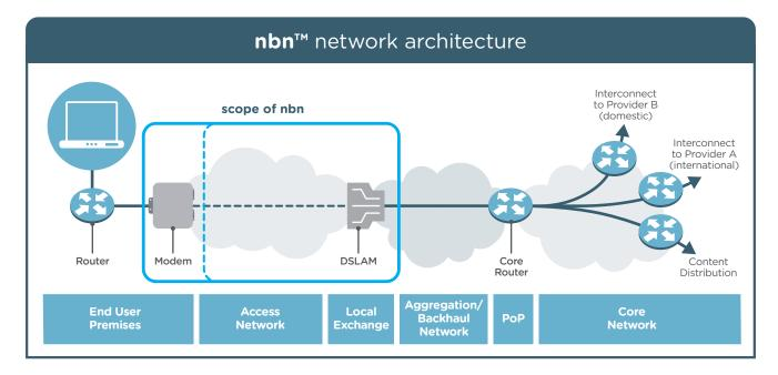
For the Service Provider, the use of **nbn**'s NEBS fibre service will see the modification, replacement or elimination of these access components, depending on the access technology:
