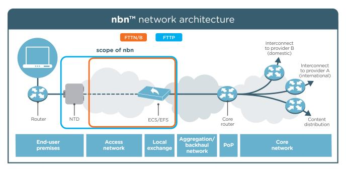
For the service provider, the use of **nbn**'s fibre-based NEBS service will see the modification, replacement or elimination of certain copper access components, depending on the access technology:
