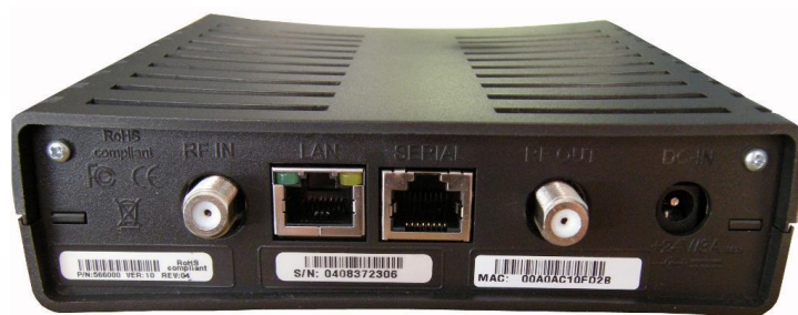
Figure 5 NTD indoor unit - back
