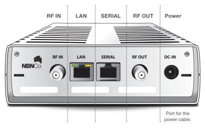
Your Network Termination Device is connected to the satellite antenna via two cables which connect to the RF IN and RF OUT connectors located at the back of your Network Termination Device.
