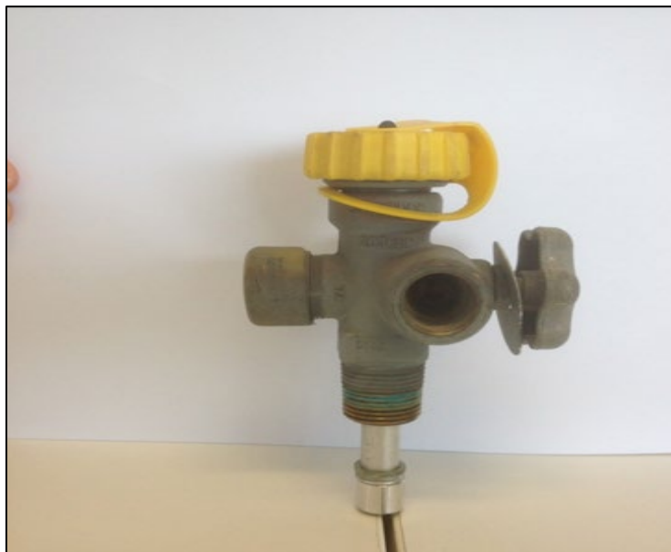
Figure 39. In-situ gas cylinder showing removable yellow cap
