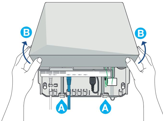
Press the two clips **A** to release the cover.
