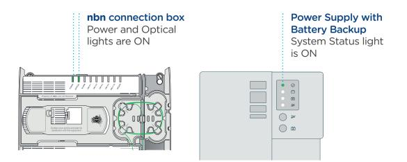
If you remove the cover from your **nbn** connection box and the lights on your **nbn** connection box or Power Supply with Battery Backup (if installed) do not match those shown in this diagram, then refer to the lights and indicators sections of this guide on pages 14–15 and 25.
